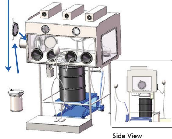
1. Shuttle Container is connected to the Operations Glovebox, the Double Doors are opened, and the waste is placed into the container. The Double Doors are closed, the Shuttle Container is removed, and the container's protective cover is installed
